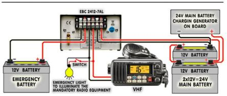
GALAXY® EBC 2412-7AL GMDSS VHF marine Class D EMERGENCY BATTERY AUTO CHARGER WIRING DIAGRAM
